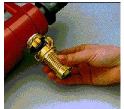
Coupling exhaust adapter for dry drilling
