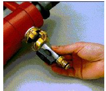
Coupling ball valve for wet drilling
